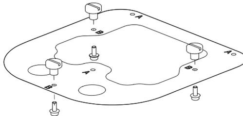
2. Fix the fixing plate to the back of the repeater with four M4 screws.
