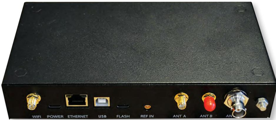
FIGURE 2: A rear view showing the connectors.
