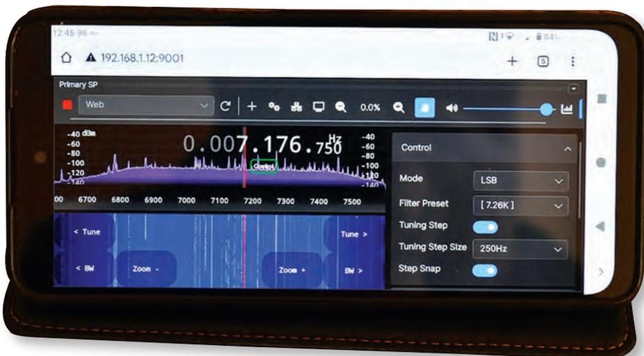
FIGURE 3: Accessing the nRSP-ST using an Android-powered Motorola G14 mobile phone.
